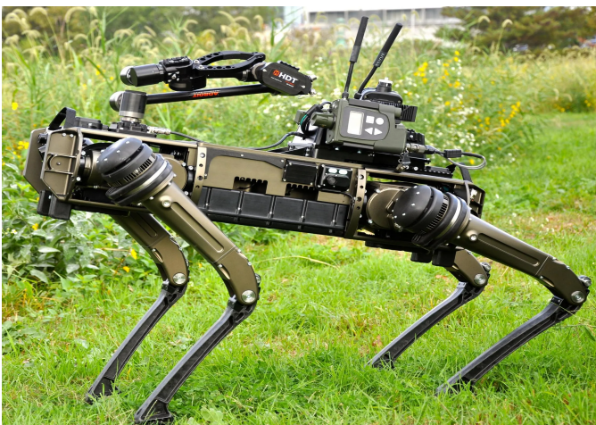
Fig. 1. A quadruped robot mounted with a 2-link manipulator and communication equipment. Reference: Photo from Google Photos https://orisalessm.live/product_details/14420612.html
